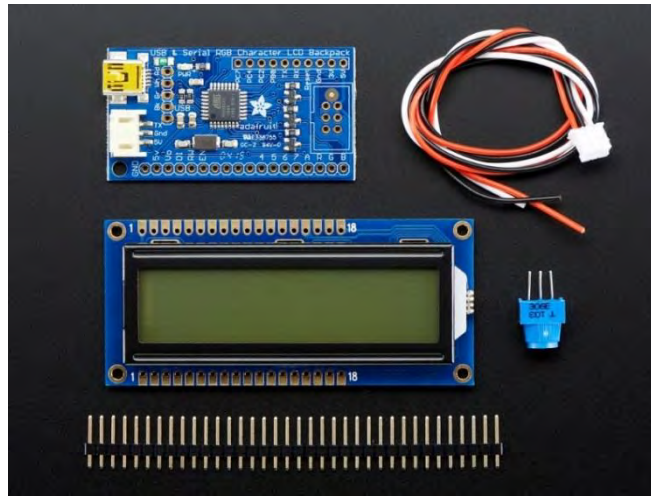
Figure 15. AdaFruit LCD and Serial Backpack.
