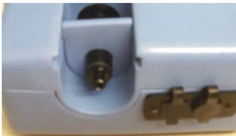
Figure 53. pDR-1500 Inlet Assembly with Total Inlet.
