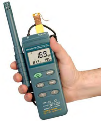
Figure 59. Handheld Temperature/RH Meter.
